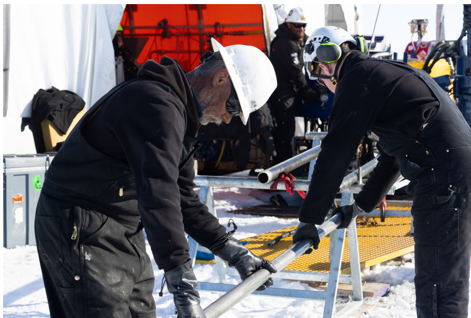
Tony Kingan (Webster Drilling) and James MacPhail (ARC) extract core splits from the drill. Photo by Ana Tovey / SWAIS2C
