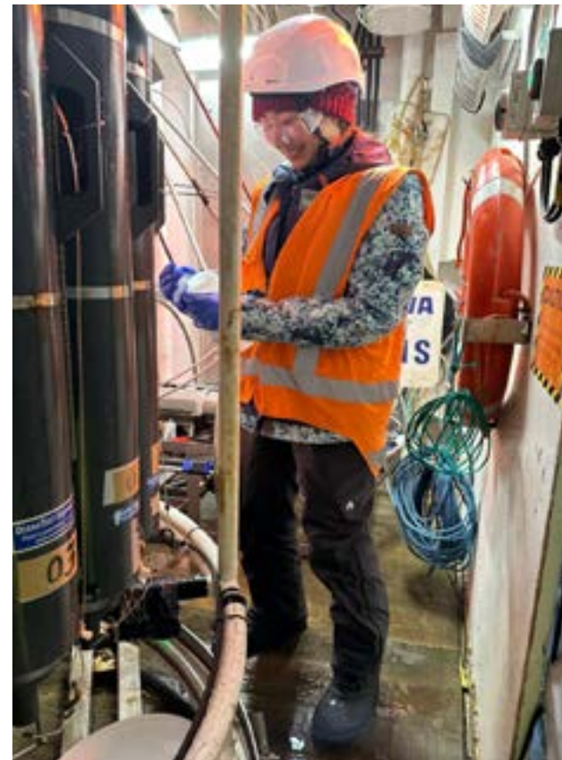
Hana onboard the RV Tangaroa, collecting seawater samples for biogeochemical analysis from the CTD rosette equipped with Niskin bottles. Photo by Denise Fernandez.
